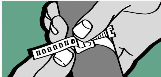
Insert band thru buckle from underneath. Pull band snug about pipe and engage serration of band on inner lug.
